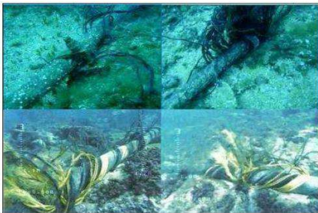
Figure 4.11: Unprotected undersea cables damaged by human activity
