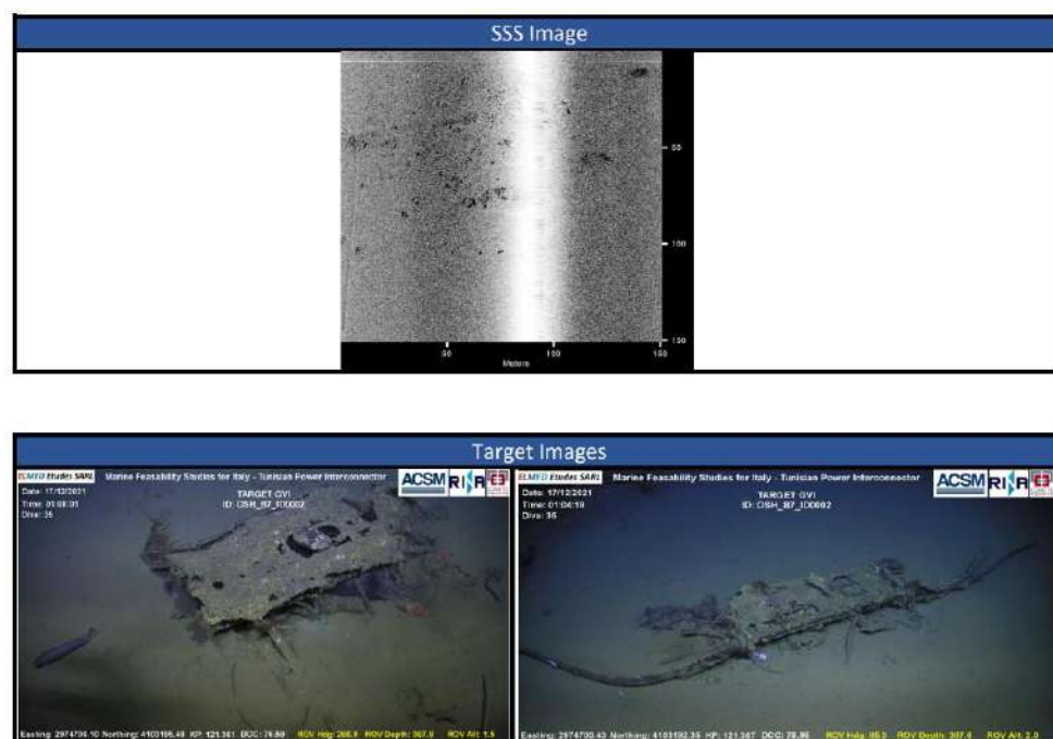
Figure 7.11: Sonar and ROV images of Historical target “Metal Debris Area OSH_B7_ID0002”
