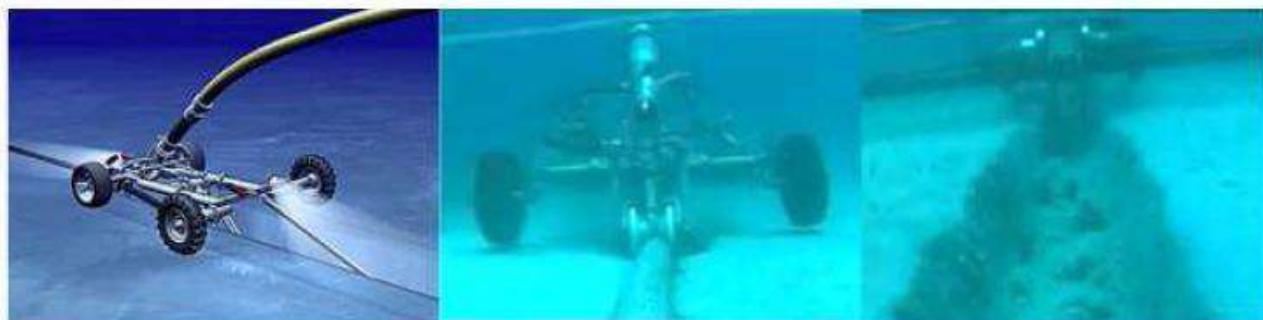
Figure 4.12: Self-propelled jetting machine
